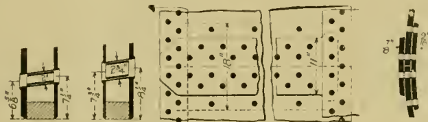
Boiler Seam and Water Space Tubes.
